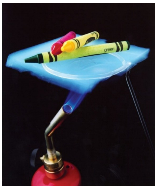
Figure 1.2: Photograph illustrating the excellent thermal-insulation properties of an aerogel
