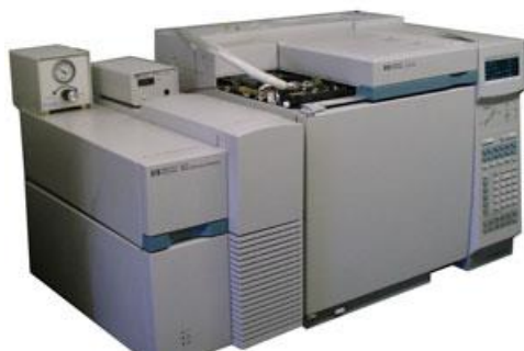
Figura 2.9. Hewlett Packard – Agilent 6890 Series GC System accoppiato ad Agilent 5973 inert Mass Selective Detector (Agilent Technologies Inc., Santa Clara, CA, USA).
