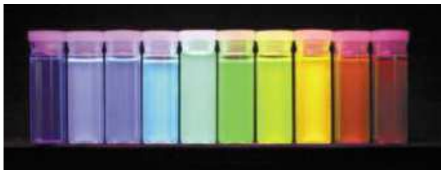
Figure 1.5 Light emission of 2(left) to 6 (right) nm CdSe dots ZnS capped excited in the UV range.
