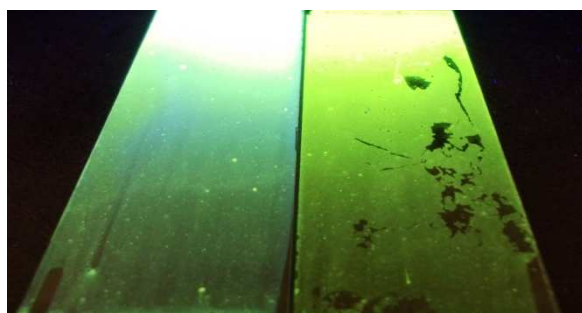
Figure 2.4 – PFLO-YG, 365nm excited coating before (left) and after (right) weathering
