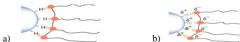
Figure 4.5 - Anchoring of a polymeric dispersant by hydrogen bonding (a) and through polarizing groups (b).
