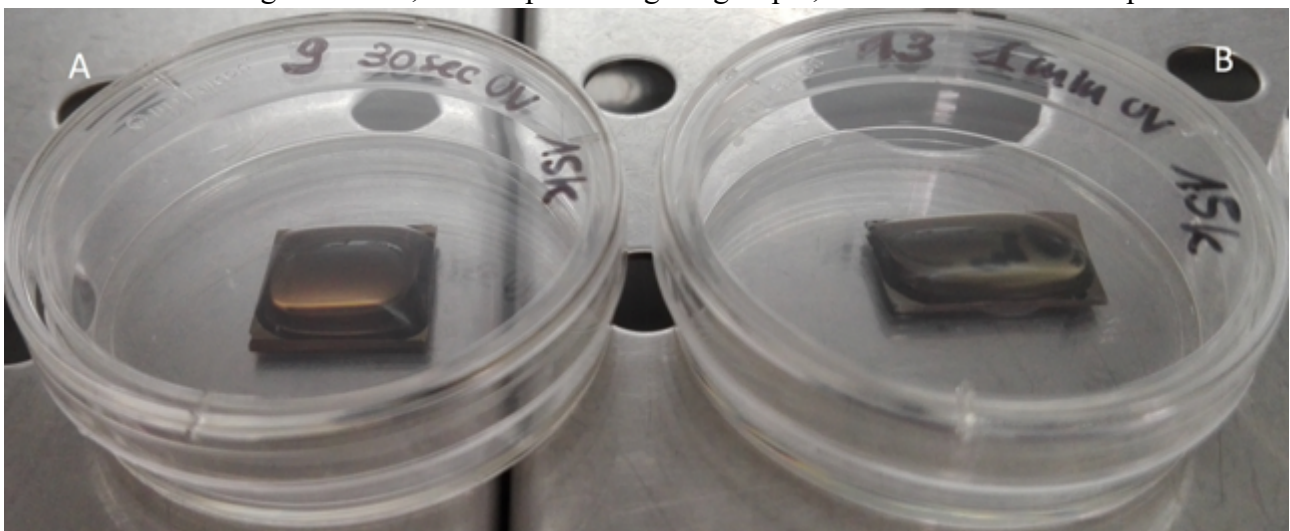
Figure 3.10. Sample A group 3 and B group 4 after poly-L-Lysine deposition, with 30 and 60 seconds UV exposition time respectively.
