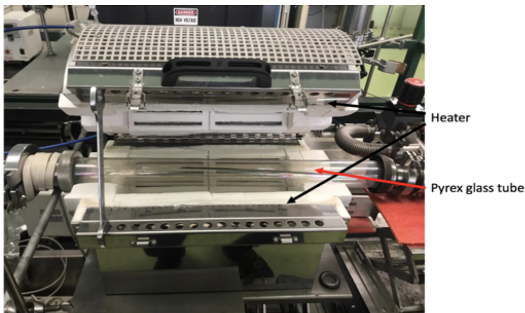
Figure 2.5. Reaction chamber of ALD apparatus used for the deposition.
