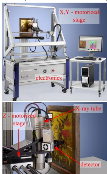
Figure 3.1 M6 Jetstream, the Bruker first model of the production run (Alfeld, Pedroso, Hommes, & Snickt, 2013).
