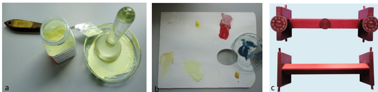
Figure 2.1 a) preparation of the pigment powder with a pestle; b) palette with the seven pigments prepared; c) film applicator
