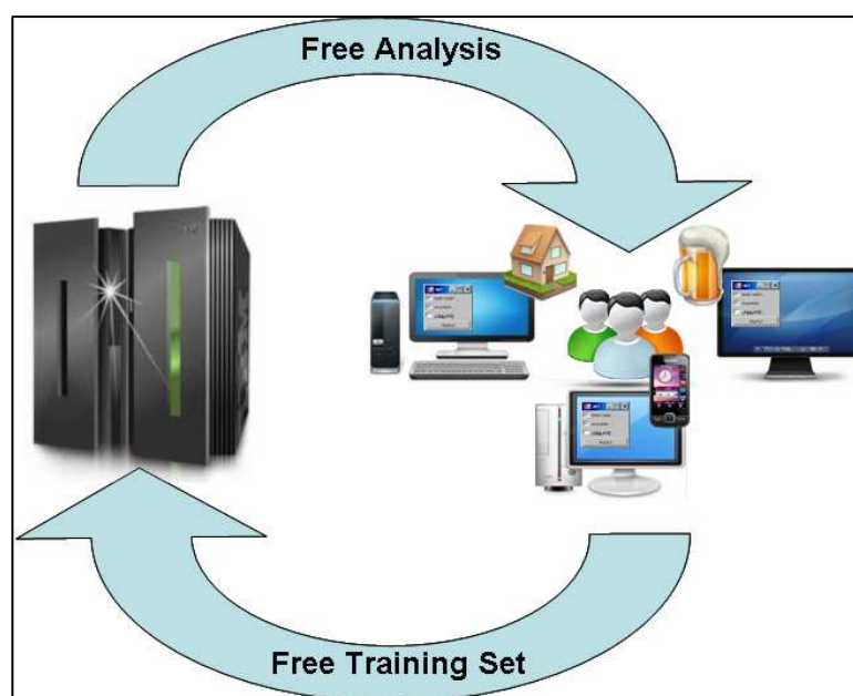
Figure 8-1: A proposed virtuous cycle that can lead to a good training set at no expense. Users on the web improve they free analysis tagging wrong records for their (local) naïve Bayesian classifier. The server saves their tagging to improve the training set.
