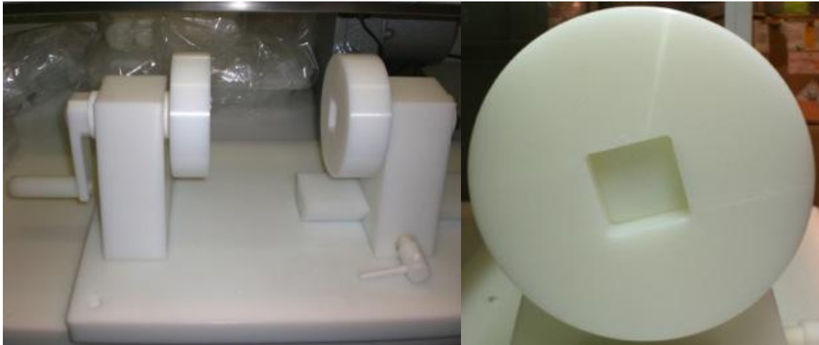
Figure 32: polyethylene turning lathe used to hold and turn the firn sections to chisel Figure 33: particular of the lathe head with a square indentation to insert the firn section (ca. 1cm deep)
