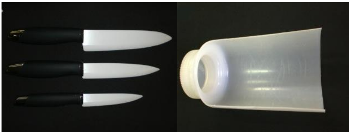
Figure 34: ceramic knives of three different sizes used to chisel the firn Figure 35: polyethylene scoop used to collect the chiselled firn
