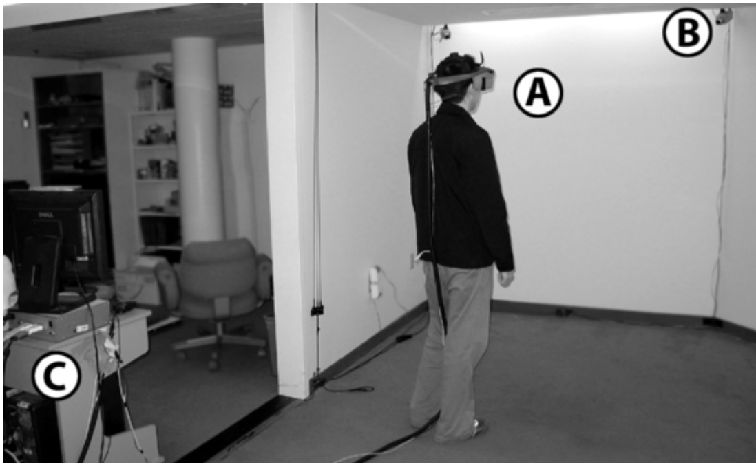
Figura 3.8. (A) head-mounted display ; (B) tracking camera ; (C) rendering machine (Yee e Bailenson, 2006).
