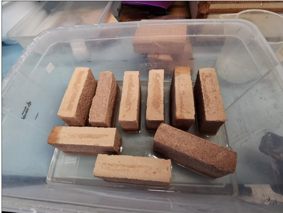
Figure 17 Samples immersed partially in NaCl oversaturated solution.
