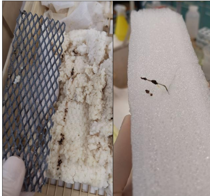
Figure 123 Acidification damages to the Ti wires.
