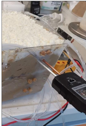
Figure 19 Holes in the container to allow pH measurements.
