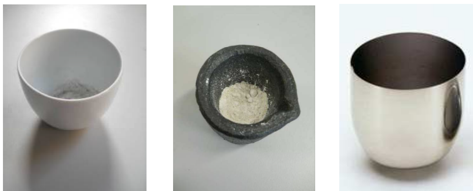
Figure 3.2 – Three type of crucible used for glassmaking: porcelain (left), silica carbide SiC (centre) and platinum Pt (right).
