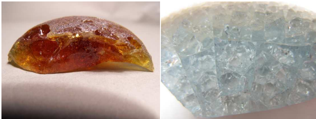
Figure 3.9 – Picture of S30 (left) and S40 (right). The first shows a brownish colour caused by Fe contamination of the glass coming from SiC crucible; the second has many cracks due to the porcelain crucible, but it is very transparent and almost without bubbles, because produced by fritting the material of S37.
