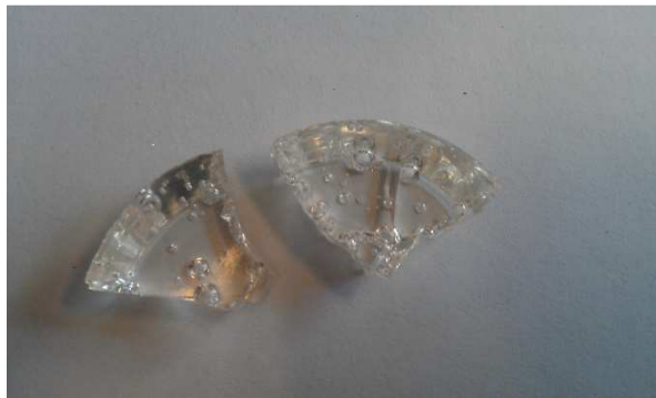
Figure 3.14 – Picture of S55, glass made into Pt crucible.
