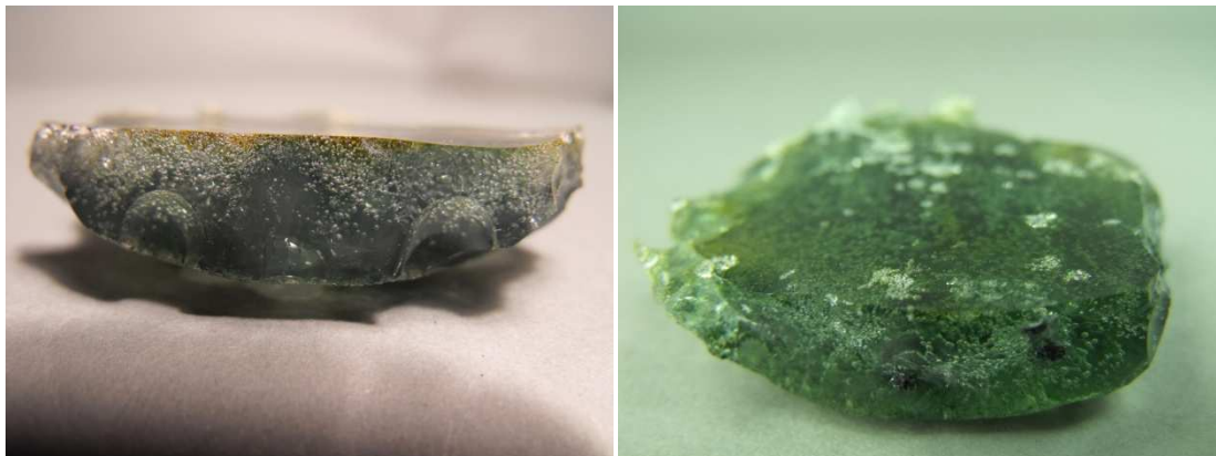
Figure 3.10 – Pictures of S31 (left) and S34 (right). The first with a bluish colour and bubbles on the top layer, the second greenish and melted at higher temperature (1450°C), that provoked the firm adhesion of pieces of crucible inside the glass.
