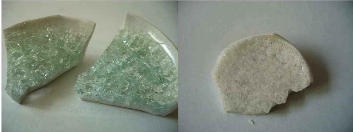
Figure 3.11 – Pictures of S46 (left) and S47(2) (right). The first, with a higher Na 2 O content, has almost no bubbles, the second has been melted at 1000°C after fritting and no glass is obtained.
