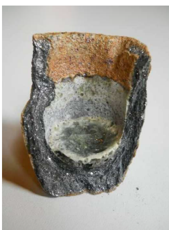
Figure 3.8 – Picture of S11, still attached to the SiC crucible. On the wall it is visible the volume change during melting.
