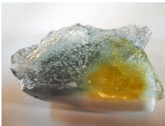
Figure 3.6 – Picture of S21 with three different layers: a transparent top layer rich of bubbles, an intermediate inner yellowish layer, a bottom crystalline and opaque layer.
