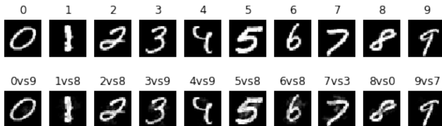
Figure 3.6: The top-side of the figure shows image of original MNIST and the bottom-side shows the perturbed images generated by ART Elastic-Net EAD(EN) attack with 100 iterations. As a result, the predicted class labels by SVM model.
