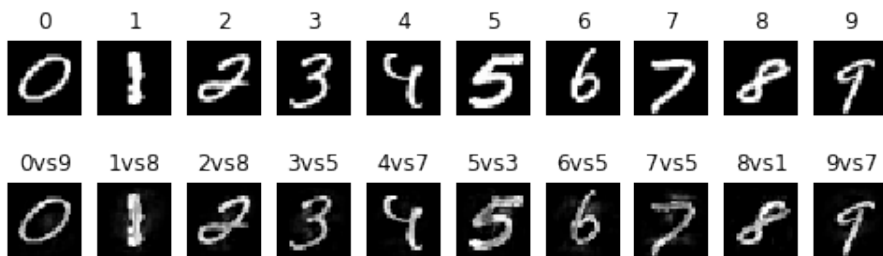
Figure 3.10: The top-side of the figure shows image of original MNIST and the bottom-side shows the perturbed images generated by ART DeepFool( \ell_2 ) attack with \epsilon = 1e - 6 and 100 iterations. As a result, the predicted class labels by SVM model.
