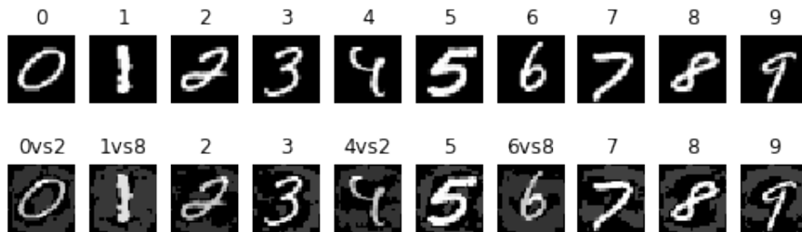
Figure 3.3: The top-side of the figure shows image of original MNIST and the bottom-side shows the perturbed images generated by ART FGSM under \ell_\infty norm bounded by \epsilon = 0.3 and predicted class labels by SVM model.
