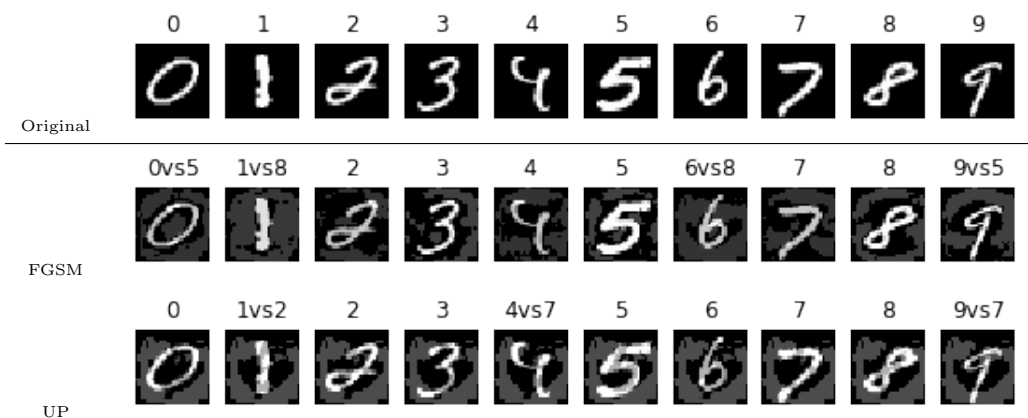
Figure 3.7: Image of original and perturbed images generated by ART FGSM and UP attack with \ell_\infty norm bounded by \epsilon = 0.3 on MNIST. As a result, the predicted class labels by SVM model.
