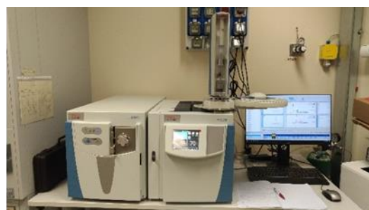
Figure 2.2 Left: Agilent Technologies 7890A GC system coupled to an Agilent Technologies 5975C single-quadrupole mass spectrometer; Right: Thermo Fisher Scientific TRACE 1310 gas chromatography coupled to a Thermo Fisher Scientific TSQ 9000 Triple Quadrupole mass spectrometer.
