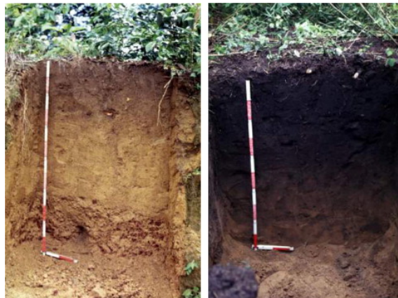
Figure 2.1: Normal Amazonian soil (left). The texture of these soils is loamy or sandy and the structure is dominated by stable micro-aggregates. The typical Terra Preta profile, the topsoils horizons have dark color and they can reach a depth up to 1 m (right) [31].
