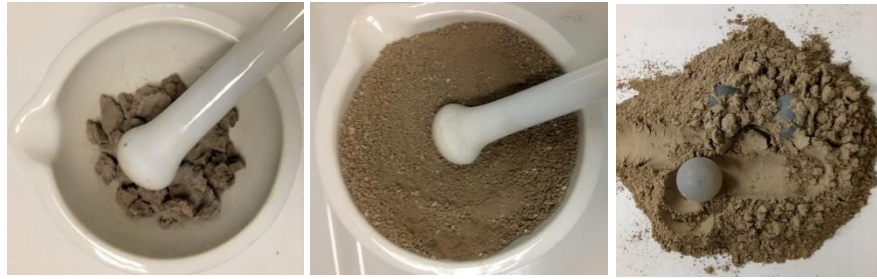
Figure 15. Soil preparation phases. From left to right: dry soil inside a mortar, soil passed through 2 mm sieve, talc-like fine dust soil.
