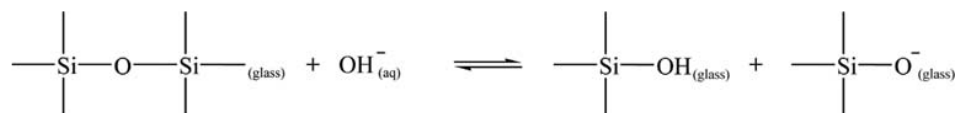
Figure 5. Stage 2 of glass corrosion. \text{OH}^- ions attack the bridges between silicon atoms, forming silanol groups and destroying the silica network [19].
