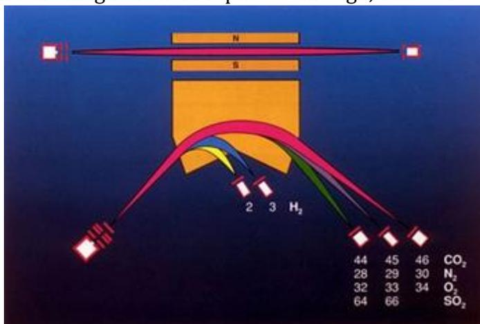
Figure 16: example image of isotope curvature due to the Lorentz force, the radius of curvature depends on the mass of the isotopes
