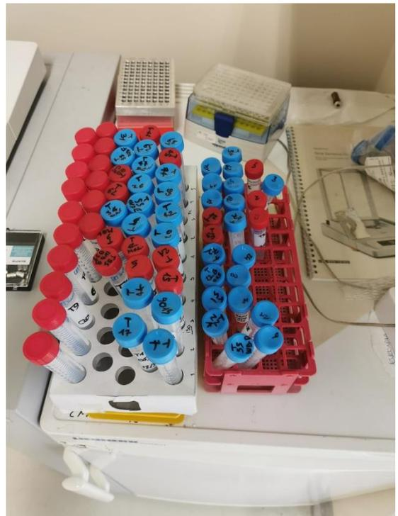
*Figure 14: the falcons containing the pulverised samples after preparation*
