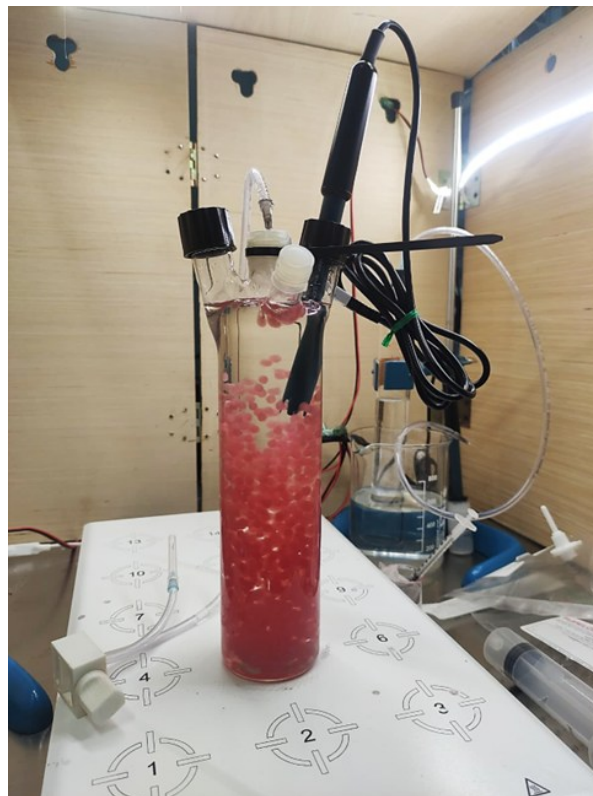
Figure 32 Column photobioreactor containing immobilized R. palustris encapsulated in alginate beads. The system was operated under anaerobic and nitrogen-limited conditions to evaluate photofermentative hydrogen production.
