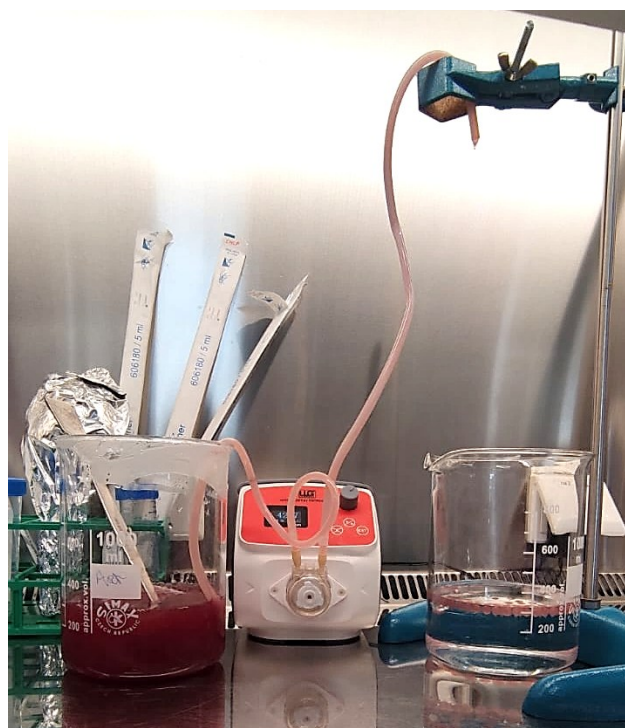
Figure 10 immobilization procedure; Dripping of the alginate solution containing R. palustris using a peristaltic pump into a CaCl 2 solution for the formation of immobilized microspheres.
