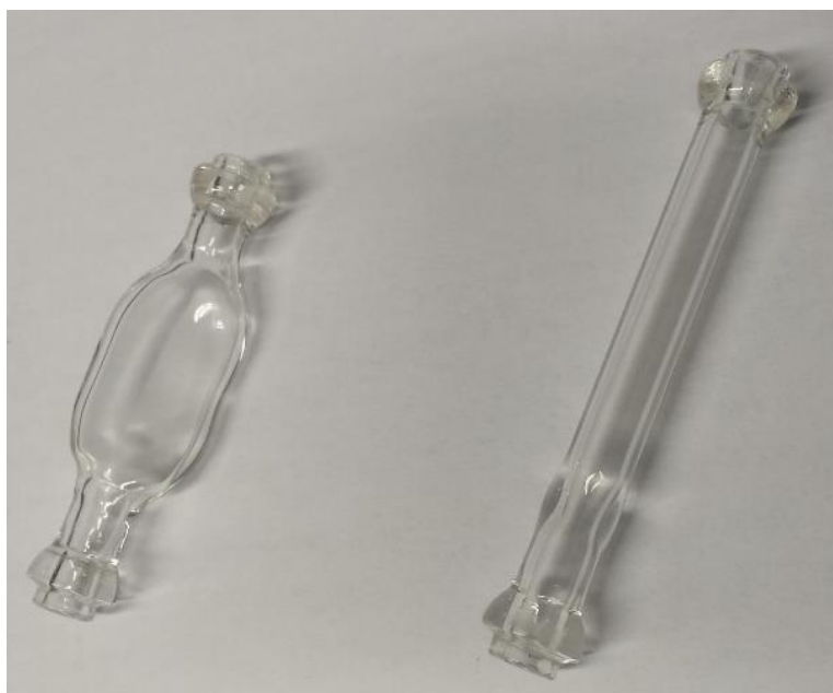
Figure 26 Plate-type thin-film photoreactor (left) and packed-bed photoreactor (right)
