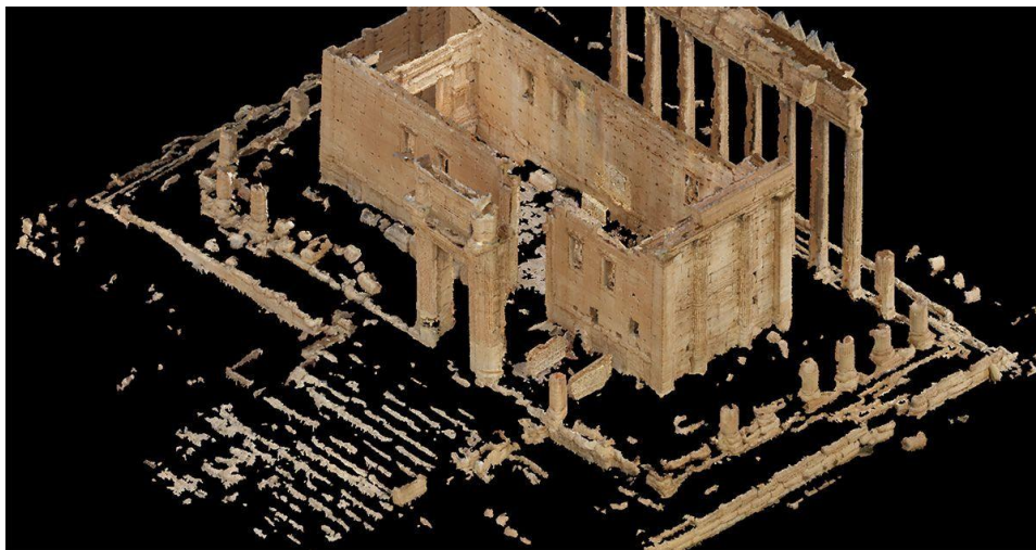
Figure 6. – Dense 3D reconstruction of the Temple of Bel at Palmyra generated from public-domain tourist photographs and professional panoramic imagery. Source: Wahbeh, Nebiker, and Fangi, 2016, ISPRS Annals of the Photogrammetry, Remote Sensing and Spatial Information Sciences , III-5, 81–88. Licensed under CC BY 3.0.
