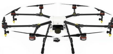
Fig. 6. Agras MG-1-DJII. Puri et al. (2017) Agriculture drones: A modern breakthrough in precision agriculture , Journal of Statistics and Management Systems, 20:4
