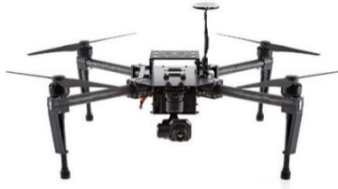
Fig. 4. DJI Matrice 100. Puri et al. (2017) Agriculture drones: A modern breakthrough in precision agriculture , Journal of Statistics and Management Systems, 20:4
