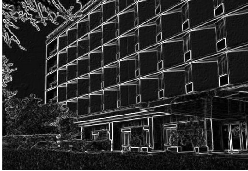
Figure 1.3: Gradient magnitude values of an image. Note that it is stronger in points where we have a large change in intensity in a particular direction.
