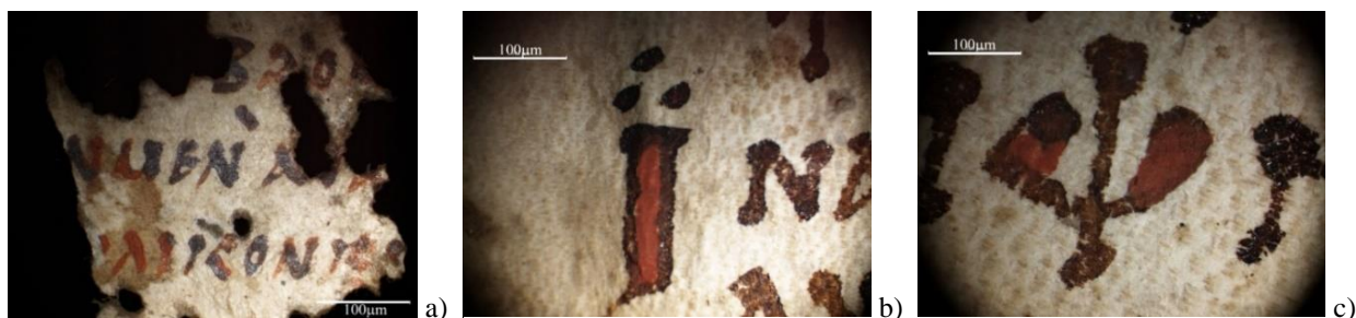
Figure 33. Red under the black ink of the fragment 20 (a) and black and red decorative letter in the folio (b and c), magnification: 16x
