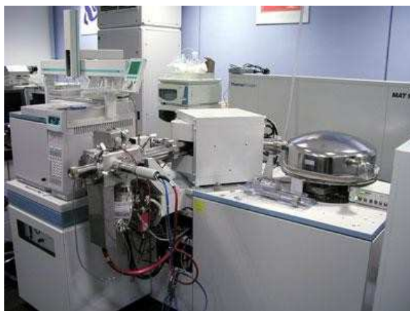
Figura 2.16: Hewlett Packard-Agilent 6890 Series GC System accoppiato a Thermo Finnigan MAT 95 XP ( Thermo Fisher Scientific , Waltham, MA, USA).
