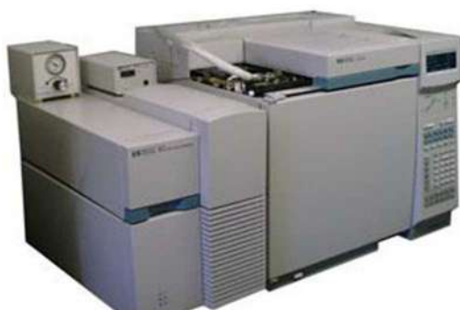
Figura 2.14: Hewlett Packard-Agilent 6890 Series GC System accoppiato ad Agilent 5973 inert Mass Selective Detector ( Agilent Technologies , Santa Clara, CA, USA).
