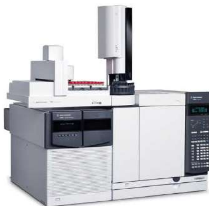
Figura 2.18: Agilent 7890B GC System accoppiato ad Agilent 7000D Triple Quadrupole ( Agilent Technologies , Santa Clara, CA, USA).
