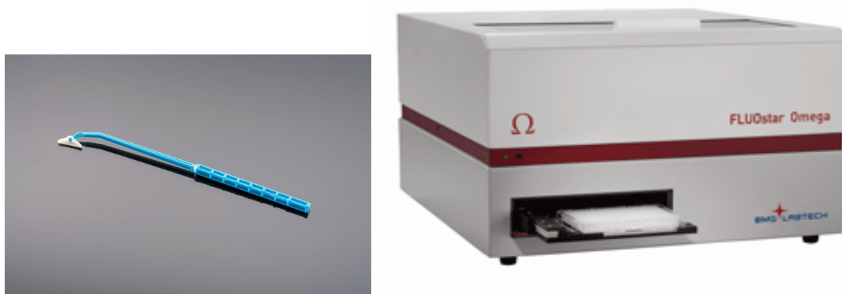
Figure 3.4.1 Example of cell scraper used for protein extraction on the left and the Spectrophotometer FLUOstar Omega used for protein quantification on the right.
