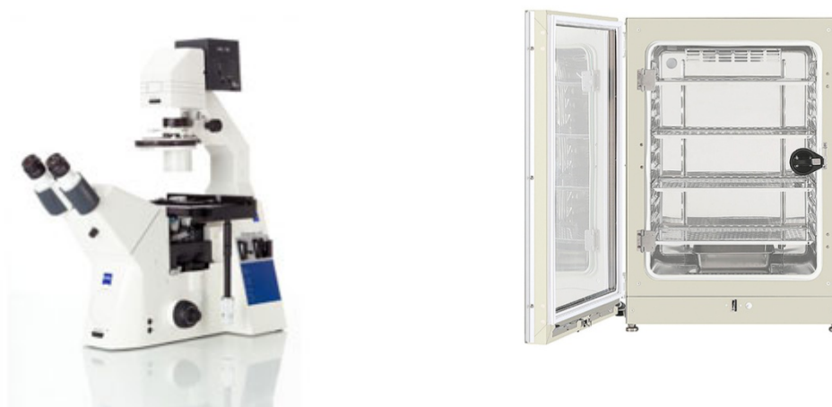
Fig.3.3.3 inverted light microscope observation (Primo Vert, Zeiss) on the left and a 5% carbon dioxide (CO 2 ) humidified incubator (Galaxy 1705, New Brunswick, UK) on the right.
