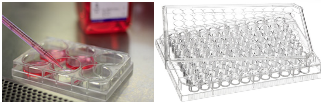
Fig.3.3.4 Example of a 6-well plate on the left and a 96-well plate in the right.
