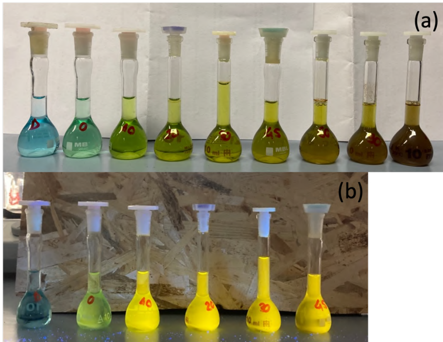
Figure 60: Methylene blue photodegraded solutions (a) taken at different time during the photocatalytic reaction, (b) irradiated by UV light.
