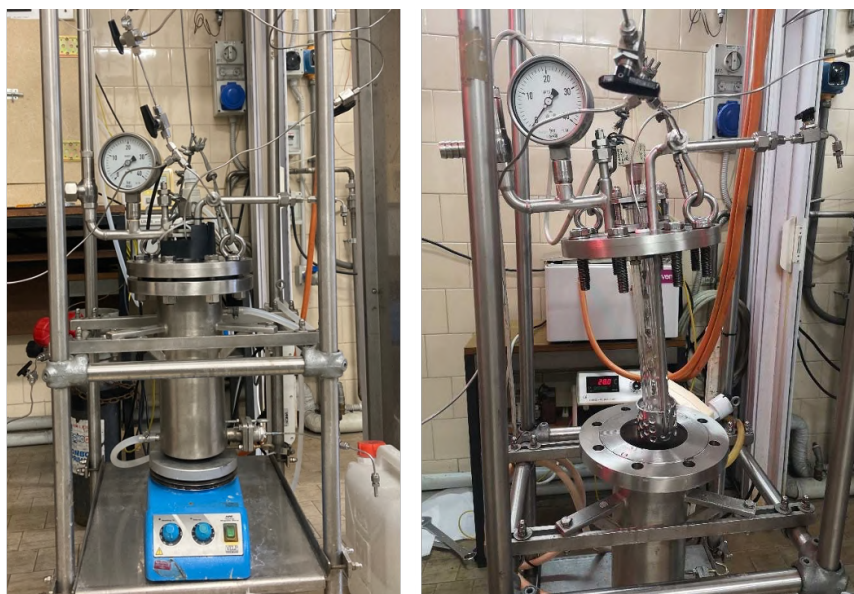
Figure 17: Liquid phase photoreduction apparatus.
