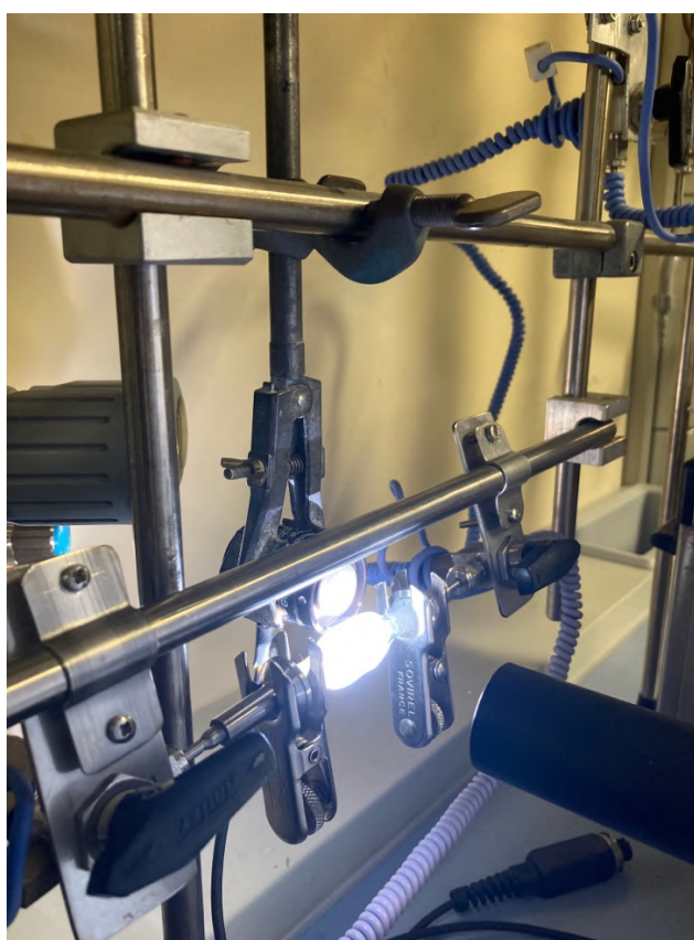
Figure 16: Gas phase reactor illuminated by solar simulator light.
