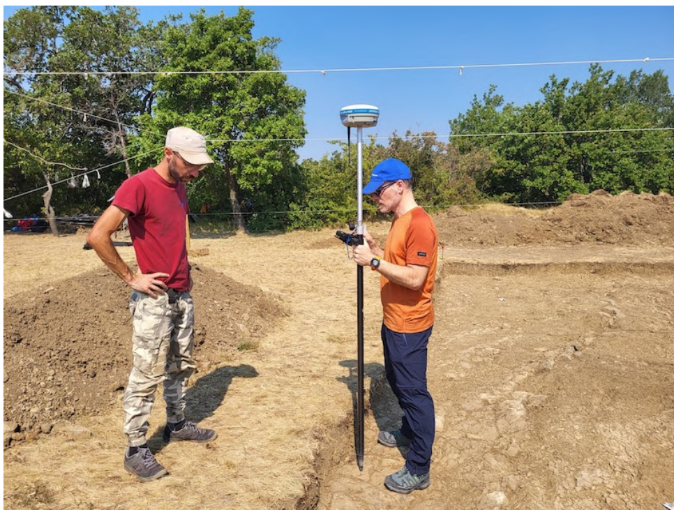
Figure 17. Differential GPS used at the Trmun site to obtain centimeter-level accuracy of location.
