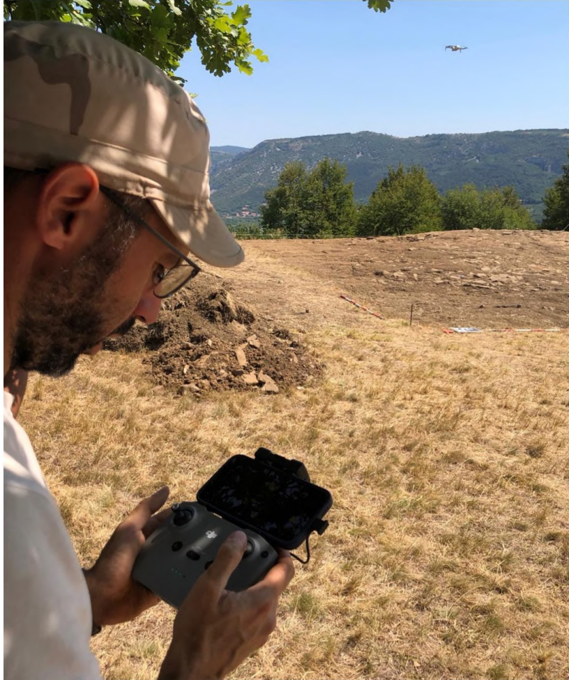
Figure 8. DJI Mini 2 drone capturing SfM photogrammetric data of the Trmun hilltop excavation in summer 2022.
