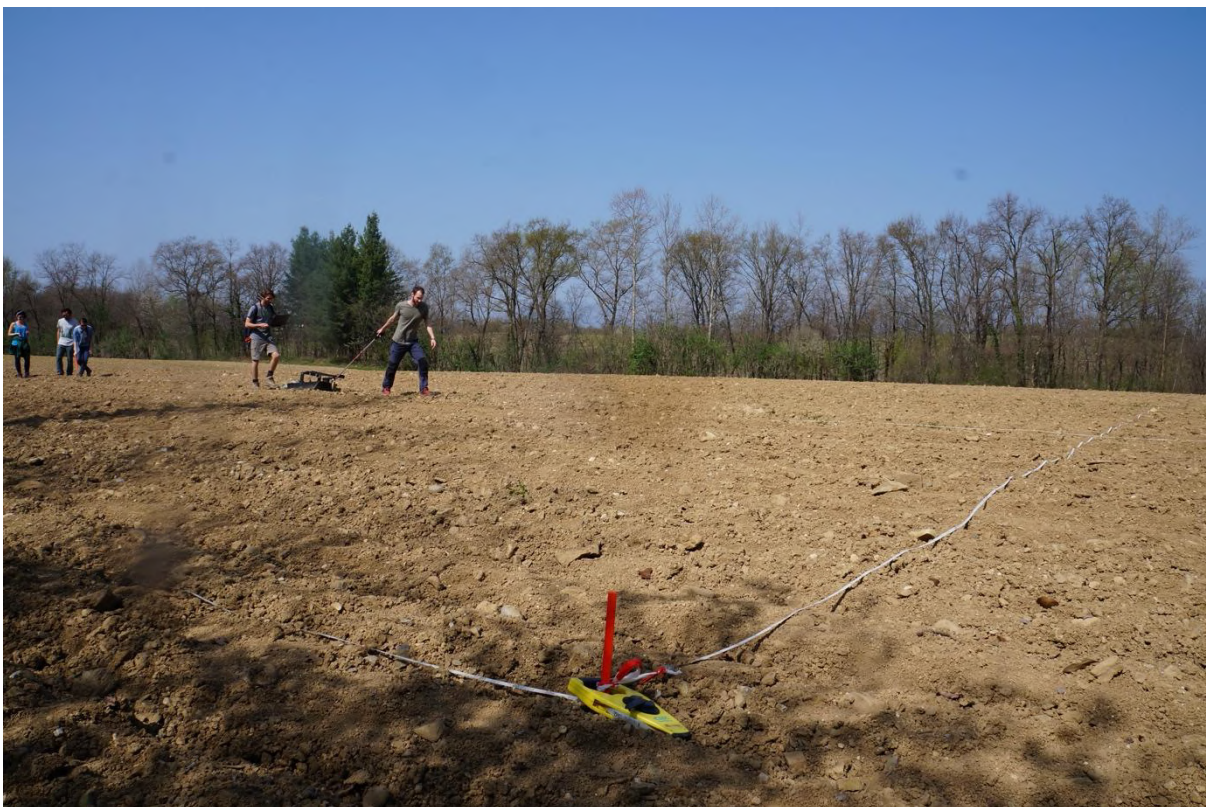
Figure 7. Example of a GPR device being pushed along a previously established grid. A surveyor walks behind the device to look at the data as it is being recorded and processed in real time. Image provided by: Forte, E., Pipan M.
