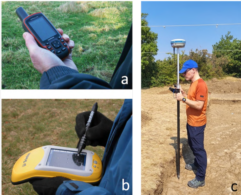
Figure 2. (a) Navigation grade device, (b) Mapping grade device, (c) Survey grade device, Differential-GPS. Note, images (a) and (b): Pearson et al., 2015.
