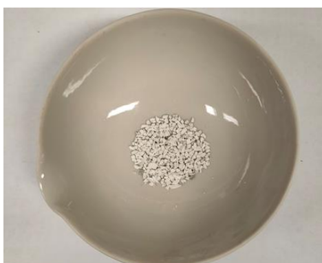
Figure 3.1: Photograph of ash residue in spider crab shell after treatment.
