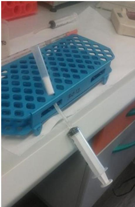
Figura 6: Cartuccia filtrante Sep-Pak® Plus Acell QMA (WATERS)
