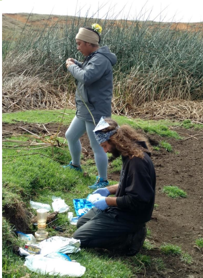
Figure 11: a) Collection of water sample from RR b) In field filtration of water samples by polycarbonate filtering system
