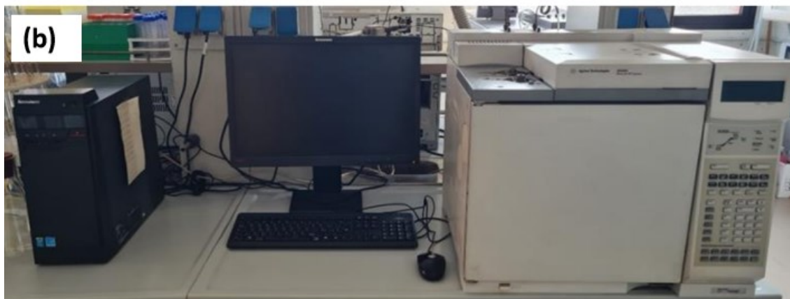
Figure 6. The (a) steam distiller used in laboratory for ammonia and TKN analysis, and (b) Gas Chromatograph used for VFA analyzes
