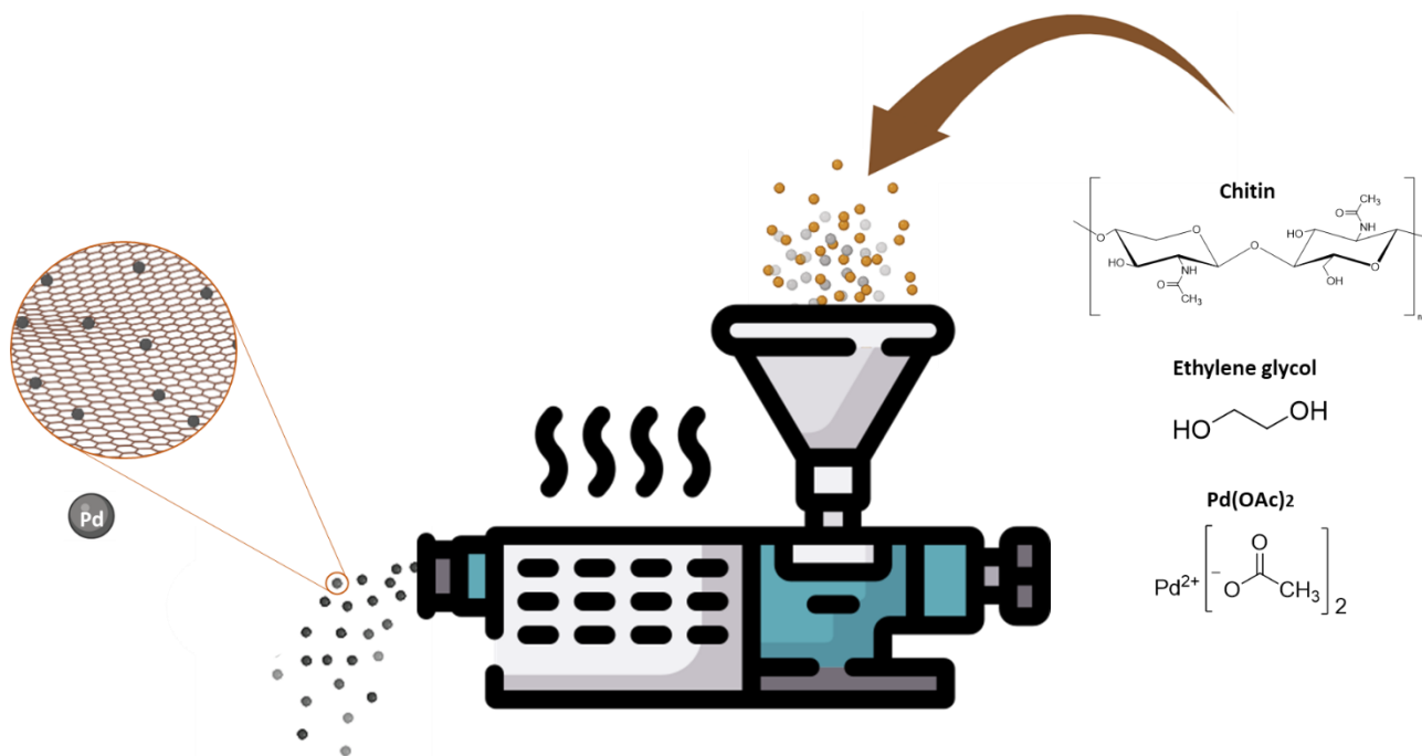
Figure 34: Schematic representation of the mechanochemically assisted synthesis of the catalytic materials.
