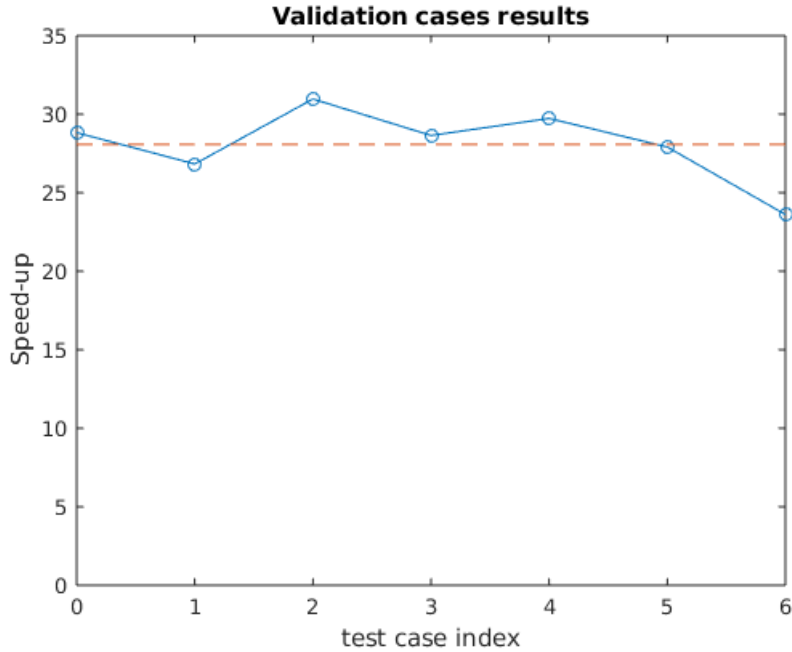
Figure 4.3: Validation test cases speed-up with a single thread. The test case index is the one reported in table 4.5. The average value is represented with a dashed line.
