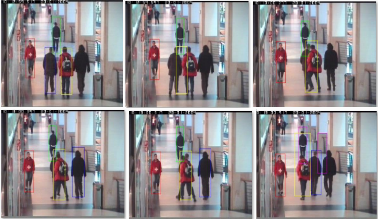
Figure. 4.10: Tracking result Re-identifying on videos with occlusion between two targets/patches
