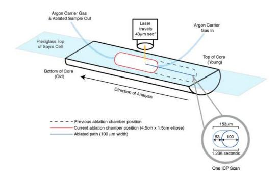
*Note.* In this case, Ar is used as a carrier gas. One ICP scan lasts 1.236 s and the laser travels with a velocity of 43 μm s<sup>-1</sup>. As a result, during one scan, the laser moves 53 μm, and with an addition of the 100 μm beam size to this value, the nominal resolution can be calculated, and it is 153 μm. Reprinted from "A New Multielement Method for LA-ICP-MS Data Acquisition from Glacier Ice Cores" by N. E. Spaulding, 2017, *Environmental Science and Technology 51*, (p. 13283).
