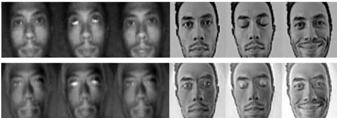
Figure 5.5.1 A subset of the training set (top), its projection and reconstruction on the face subspace (bottom)
