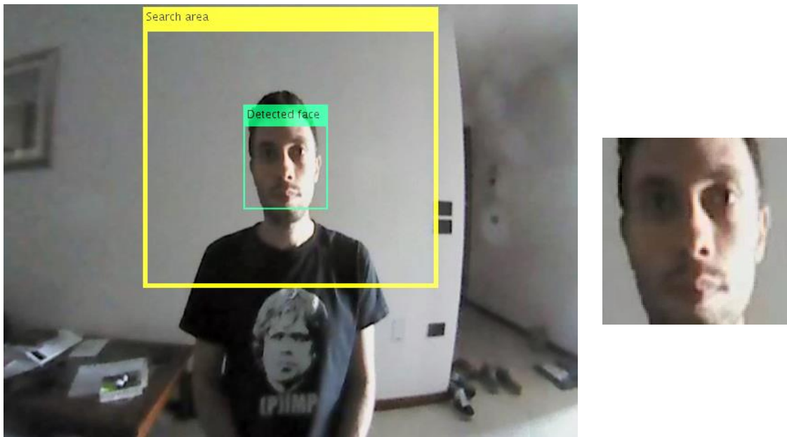
Figure 5.3.1 Face detection example, with search area and detection area (left), and detected face (right)
