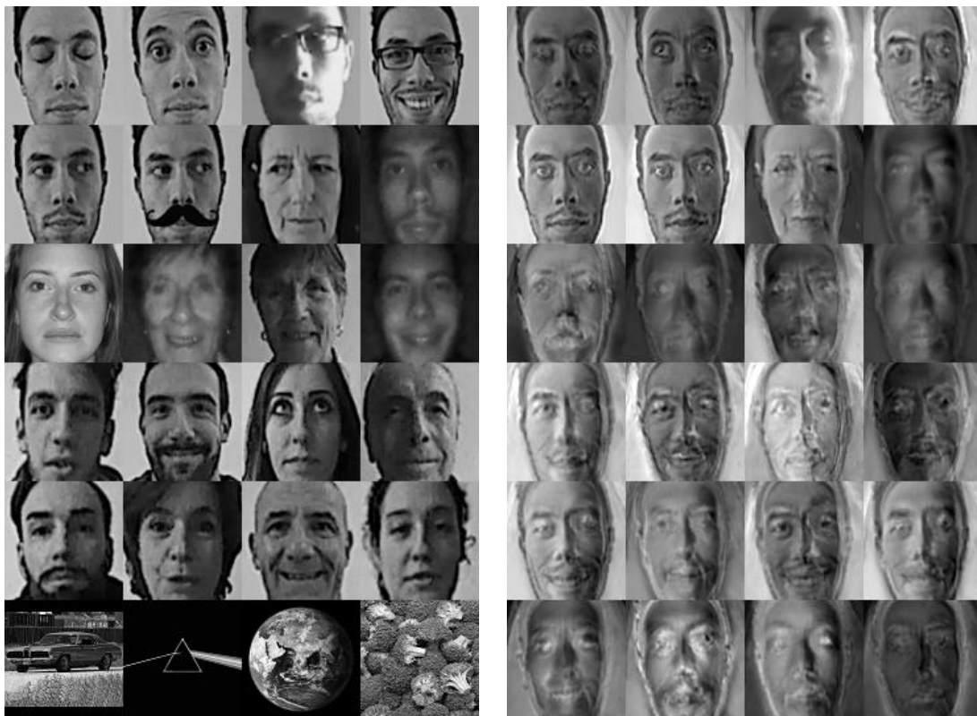
Figure 5.6.1 - Some test set images (left) and their reconstruction in the face subspace (right) using the first 30 eigenvectors
