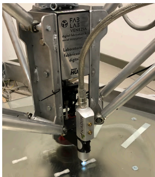
Figure 14. Plasma torch installed on the printhead.
