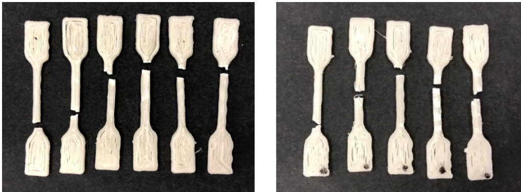
Figure 27. Six non-treated samples (left) and five treated sample (right) after tensile tests.
